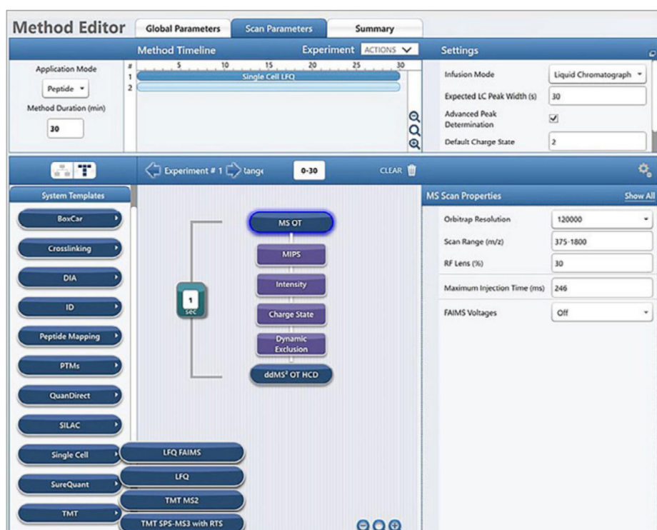
Figure 3. Orbitrap Ascend Tribrid MS intuitive method editor features a drag-and-drop user-friendly interface with predefined, optimized method templates for a wide range of applications. This allows scientists to generate high-quality data easily for applications including single cell proteomics, PTMs, TMT multiplexed quantitation, Data-independent Acquisition (DIA), Metabolomics, Lipidomics, Native protein characterization, and Thermo Scientific™ SureQuant™ methods and more.
