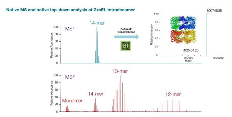
Native MS1 analysis of the GroEL tetradecamer protein complex, a molecular chaperone required for the proper folding of many proteins in cells. Using in-source trapping, very efficient desolvation and fragmentation of the GroEL 14-mer into monomer and stripped complexes (13-mer and 12-mer) is achieved.
