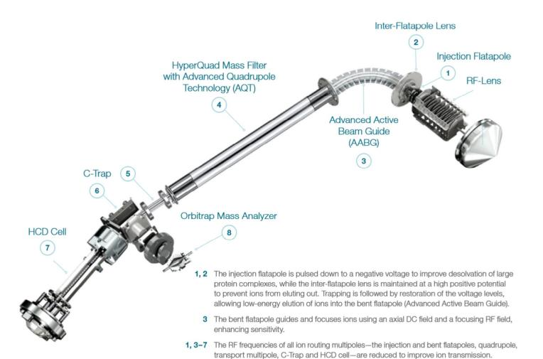
8 High mass ions are efficiently injected into the Orbitrap mass analyzer by adjusting the slew rate of the high-voltage pulse that captures ions in the analyzer.
